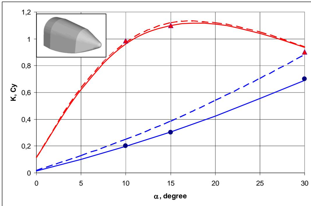
Figure 1: The aerodynamic coefficients  $K$  (red lines and triangles) and  $C_y$  (blue lines and circles) for the descent vehicle type lifting body
