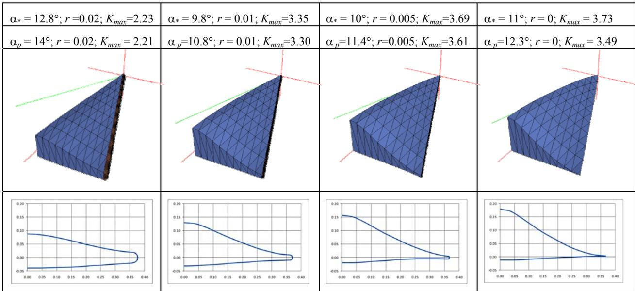
Figure 5: Shapes and  $K_{max}$  values for delta wings ( $V \approx 0.028, \chi = 70^\circ$ ) with blunted leading edge.  $M = 10, C_f = 0.002$
