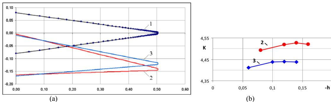
Figure3: Cross sections of the initial (1) and optimal wings and lift-to-drag of these optimal wings; ideal gas – red (2) , tangent wedge – blue (3)
