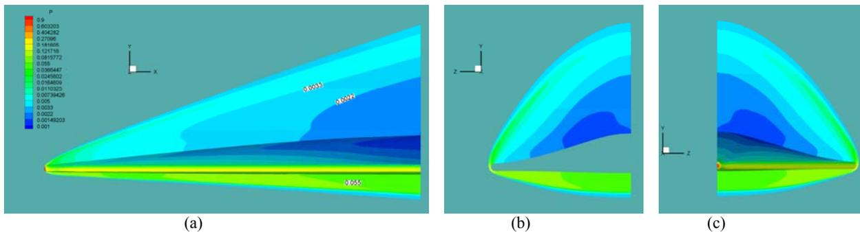
Figure 2: Flow patterns around the delta wing
