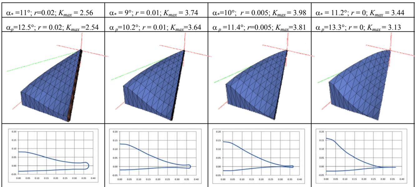
Figure 4: Shapes and  $K_{max}$  values for delta wings ( $V \approx 0.028, \chi=70^\circ$ ) with blunted leading edge.  $M=6, C_f = 0.002$
